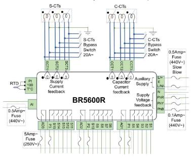
The protection fuses and switches shown in diagram above should be external to BR5600R controller. Users are expected to take care of this requirement for adequate protection to unit and system.
